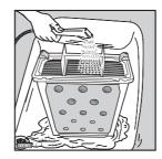
Clean it with a brush and rinse it under the shower if necessary. Also clean the outside, removing all fluff. Clean the rubber seal round the condenser cabinet and in the inner part of the small door with a damp cloth..
